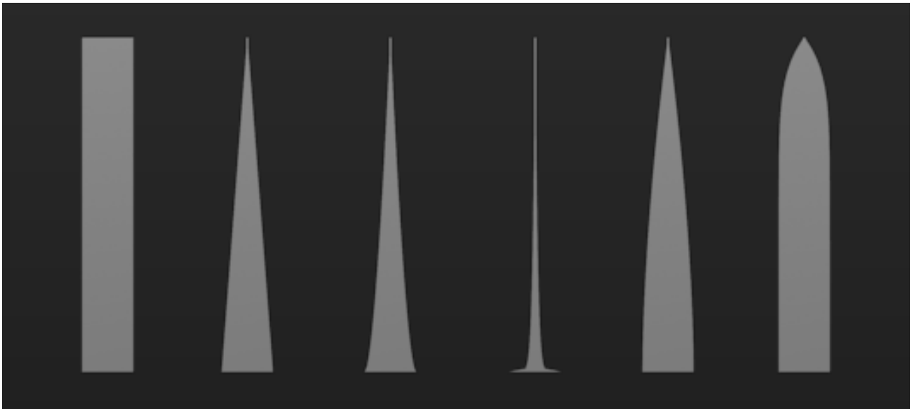
Fig. 2.1499: Various Shape settings. From left to right, 0 (root and tip are equal in the first), 0, -0.4, -0.9, 0.4, 0.9.
