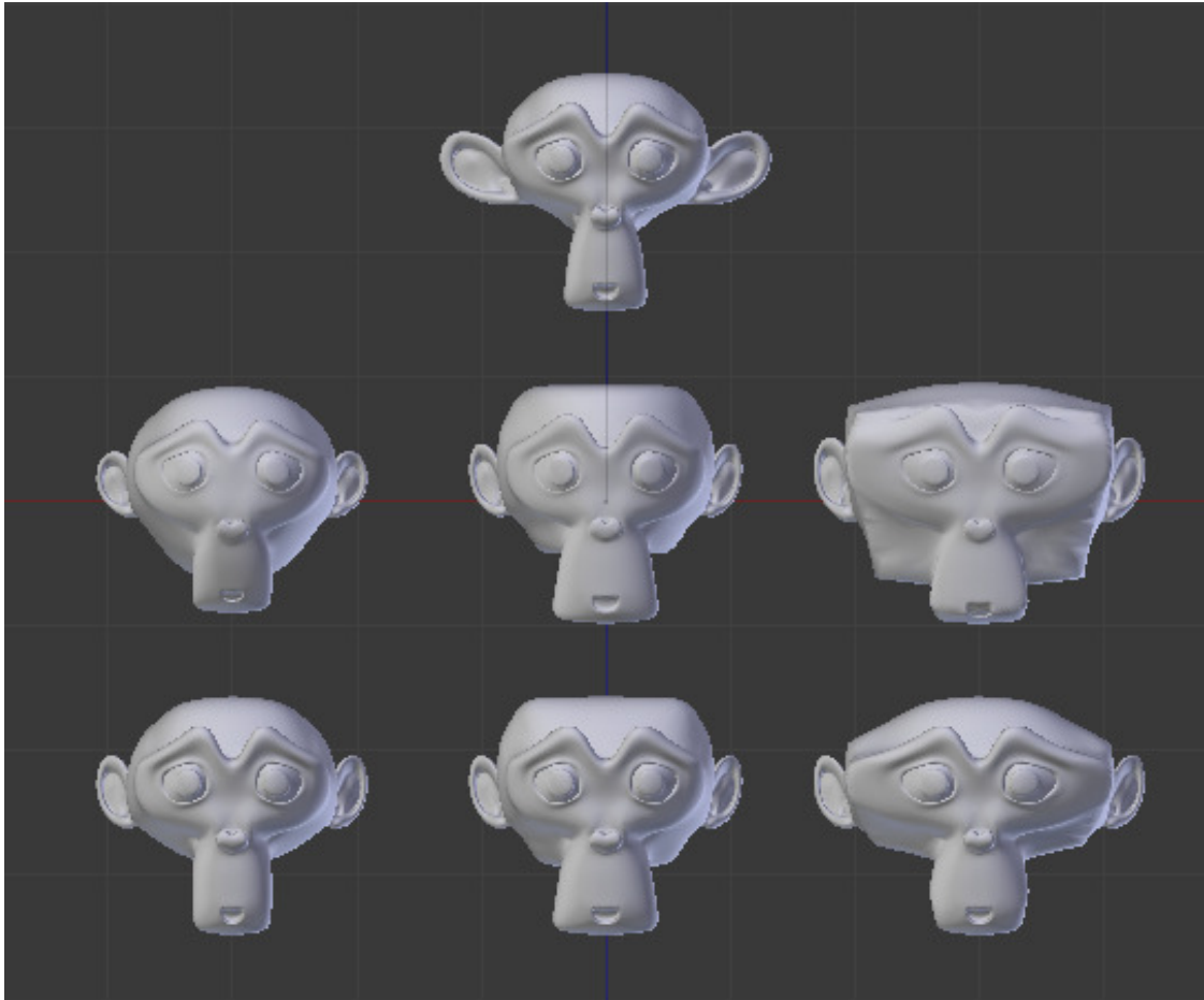
Fig. 2.860: Top: Suzanne without modifiers. Middle: Suzanne with each type of Cast Modifier (Sphere, Cylinder and Cuboid). Bottom: Same as above, but now only X axis is enabled. Sample blend-file .
