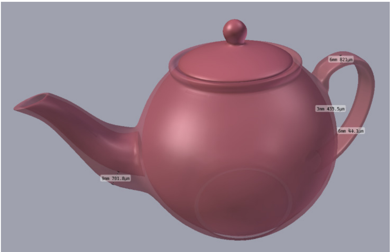
Fig. 2.47: Example using the ruler to measure thickness.
