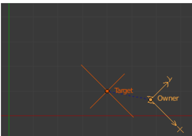
Fig. 2.1044: Offset cleared. Clear Inverse has been clicked. Owner is fully again controlled by Target_1.
