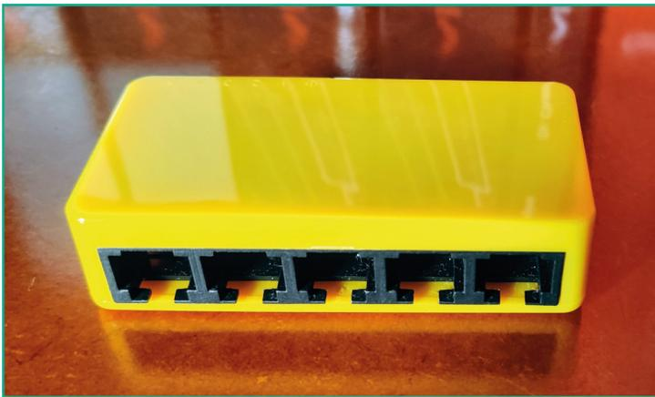
Figure 17.6 – USB-powered network switch
