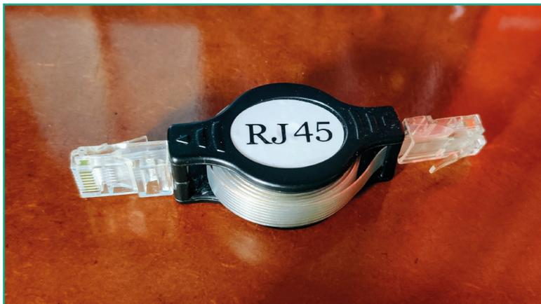
Figure 17.7 – Retractable cable
